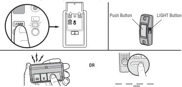
The garage door opener lights will flash (or two clicks will be heard) when the code has been programmed. Repeat the steps for programming additional remote controls or keyless entry devices. If programming is unsuccessful, follow the steps to program using the garage door opener LEARN button.
