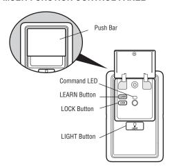
SYNCHRONIZE THE DOOR CONTROL: To synchronize the door control to the garage door opener, press the push bar until the garage door opener activates (it may take up to 3 presses). Test the door control by pressing the push bar; each press of the push bar will activate the garage door opener. PUSH BAR: Press the push bar to open or close the door. LEARN BUTTON: Use to program compatible remote controls, wireless keyless entries and myQ® devices to the garage door opener.
