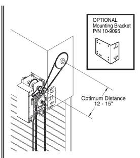
**IMPORTANT:** The shelf or bracket must provide adequate support, prevent play between operator and door shaft, and permit operator to be fastened securely and with the drive shaft parallel to the door shaft.
