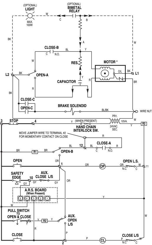
\* TO REVERSE MOTOR ROTATION INTERCHANGE RED AND YELLOW MOTOR WIRES.
