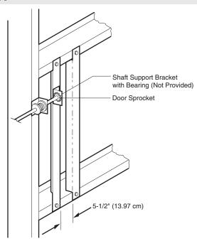
All MJ, MH, and HMJ series operators have dual output shafts and may be mounted on either the right (standard) or left side of door, and in either a vertical (standard) or horizontal mounting position. If you need to move the drive sprocket, loosen BOTH set screws, remove the sprocket and key, and place on the opposite side of the drive shaft. Be sure to tighten BOTH set screws securely
