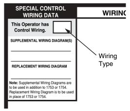
Wiring Diagram label on inside cover of electrical box
