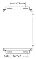
NOTE: An external stepdown transformer is used for the 460V/575V operator incoming MAINS voltage. Dimensions of the stepdown transformer are the same as the controller.
