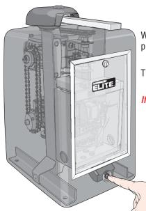
When the gate operator's audio alarm (see below) has been tripped, the reset switch must be pushed for the operator to function again.
