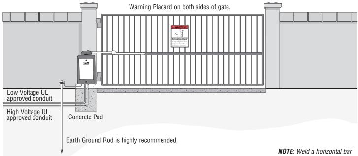
**NUIE:** Weld a horizontal ball across entire gate on any installation for strength.
