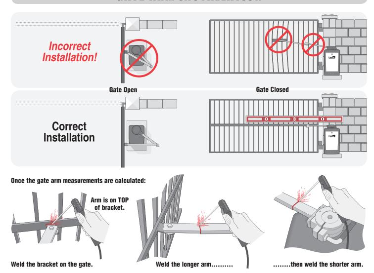
Completely weld around the rectangular tubes and bracket!
