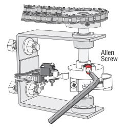
Loosen screws to turn limit cams.
