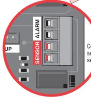
Connect both edge sensors parallel to sensor connector.
