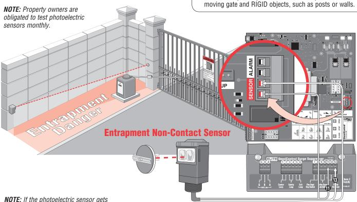
**NOTE:** If the photoelectric sensor gets blocked while the gate is closing, it will stop and reopen. The gate will remain open until the obstruction is cleared.
