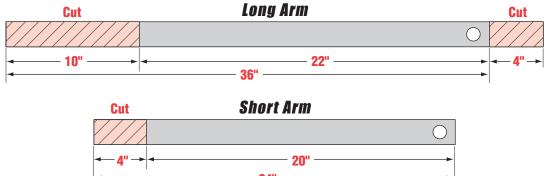
Follow the exact measurements, then cut the standard arm to meet the shorter measurements.
